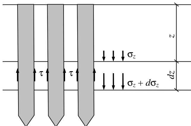
Fig. 3. Diagram of load action in the foundation base layer of thickness  $dz$
