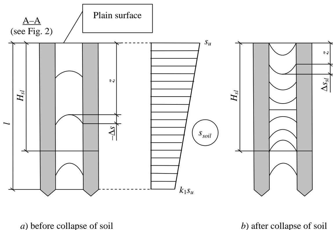
Fig. 1. Plots of mutual displacement of soil and piles
